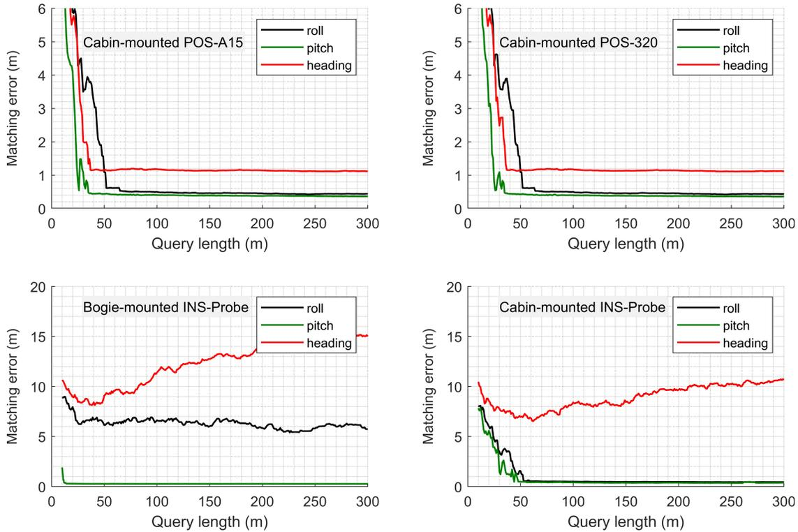
Fig. 9. Matching errors (root mean square) as a function of the query subsequence length using the roll, pitch and heading responses.
