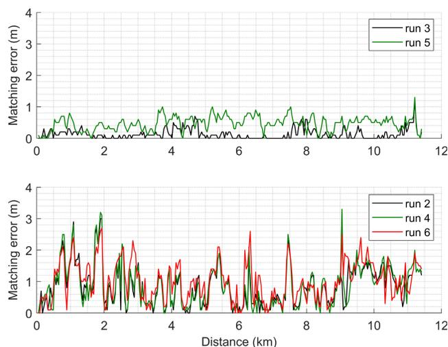
Fig. 8. Matching errors (absolute value) using the pitch profile with a query length of 100 m from POS-320. The pitch angle measurements from run 1 were used as the map.
