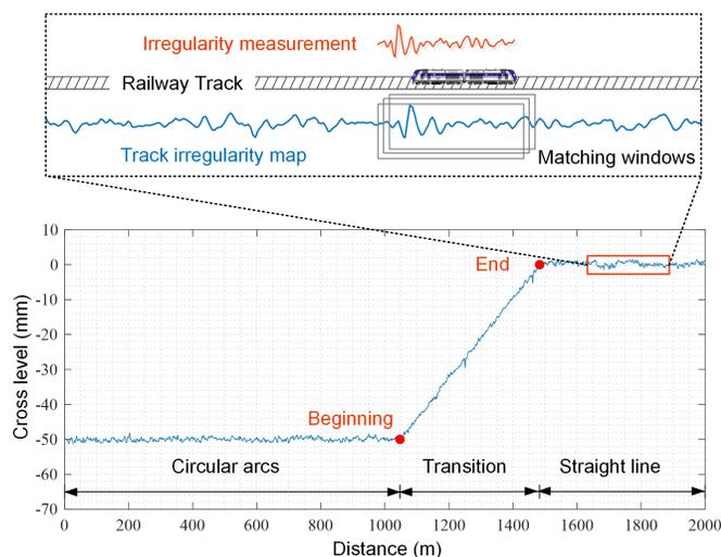
Fig. 1. Concept of train localization by matching a track irregularity profile, taking the cross level as an example, to an onboard digital map.
