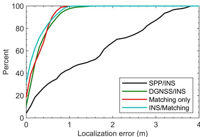
Fig. 14. Cumulative distribution function plots of the localization errors of different methods using POS-320.
