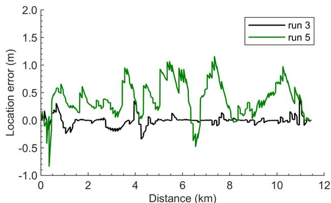
Fig. 12. Localization errors of the INS aided by pitch profile matching from POS-320.
