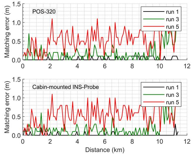
Fig. 10. Matching errors (absolute value) using pitch angle with a 100 m query length. The background map comes from the solutions of POS-A15 in run 1.
