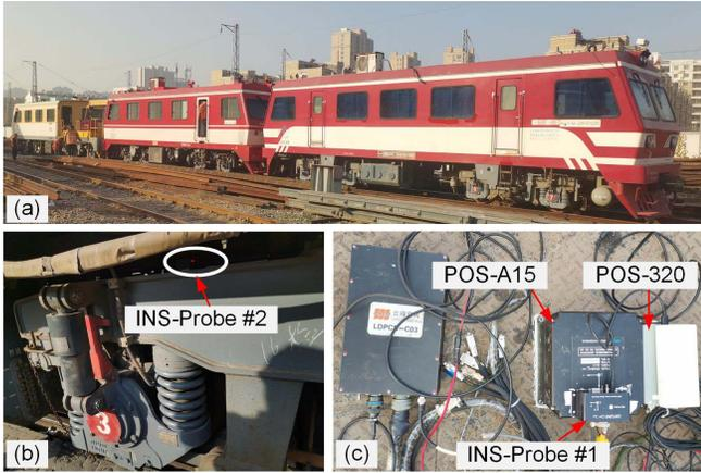
Fig. 3. Photograph of the experimental setup. (a) Overview of the main-tenance train; (b) MEMS IMU mounted on the bogie platform; (c) IMUs mounted inside the cabin.
