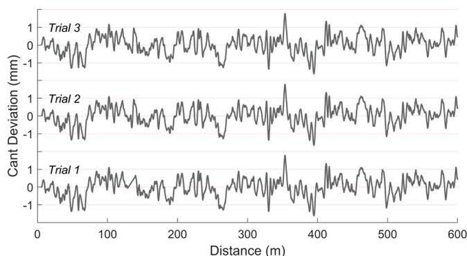
Fig. 2. Typical plots of the cross-level deviation measurements in three independent surveys over the same slab track section.
