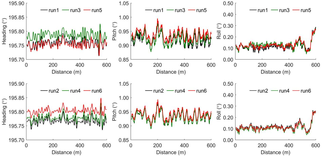
Fig. 7. A typical section of the attitude measurements from the cabin-mounted POS-320 as a function of the path distance over 6 runs.
