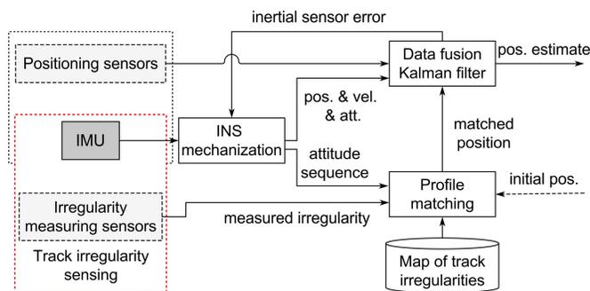
Fig. 11. Concept of the train localization prototype based on track geometry feature matching.
