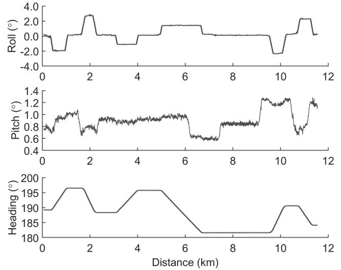
Fig. 6. Typical attitude responses of the cabin-mounted POS-320 with respect to the travel distance.
