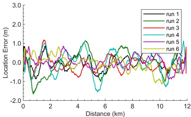
Fig. 13. Localization error of the DGNSS/INS integrated solution from POS320.
