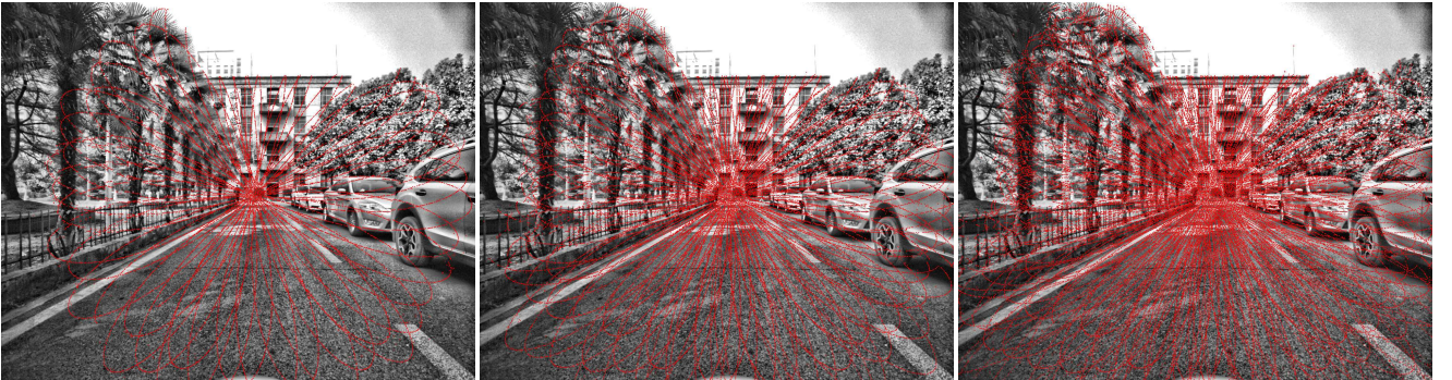
Fig. 4. The projected point clouds in the image plane (the robot is in dynamic condition with a speed of about 1.5 m/s). Each point is expressed as a red cross for better visualization. The accumulation time for the three images are 0.25 second (left), 0.5 second (middle), and 1.0 second (right), respectively.
