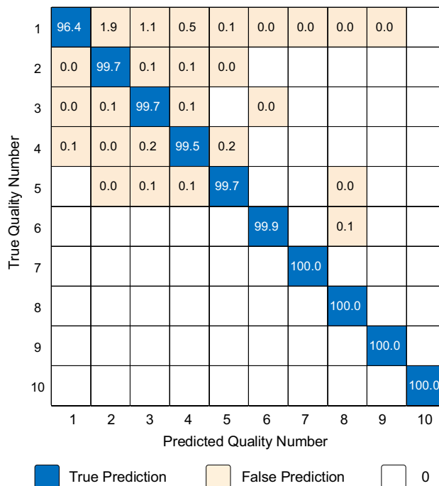
Fig. 3 Confusion matrix for using the CART-Bagging algorithm. The values are in percent
